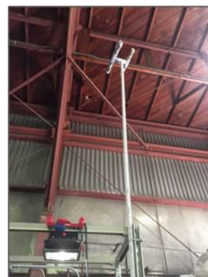
Aegis 400's sensors elevated to monitor rising gases.
